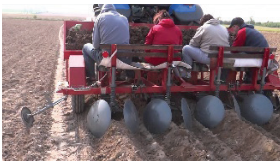
Picture 6 Miscanthus mechanical planting with three-row planter
