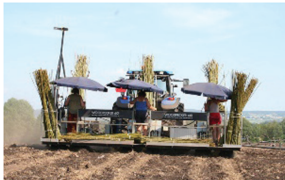
Picture 2 Salix mechanical planting with three-row planter
