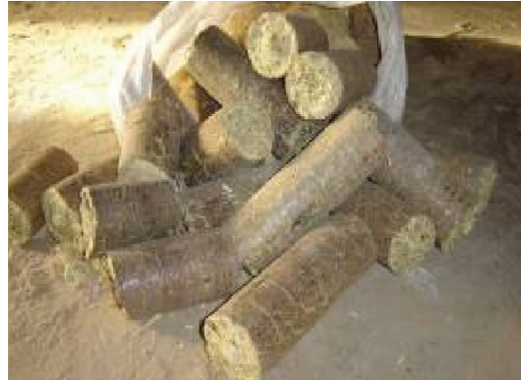
Picture 19 Straw briquettes from a hydraulic press
