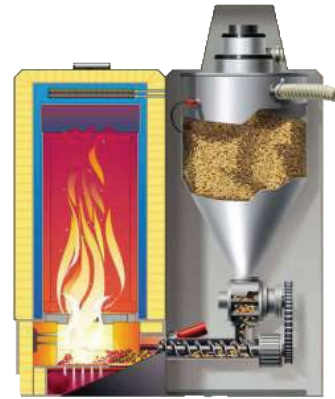
Picture 10 Pellet boiler functioning principle
